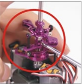
9. 调整倾斜盘和下中心座组位置与伺服器摆臂平行即可 Adjust the swashplate and bottom central holder set, make it parallel with the servo horn.
