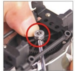
12. 齿轮固定环锁紧主齿轮 Lock up the main gear with the gear retainer ring.
