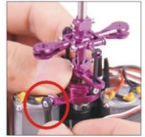
8. 伺服器摆臂上的拉杆头与倾斜盘连接 Connect the push-rod on the servo horn with the swashplate.
