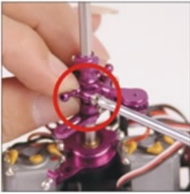
5. 夹头片装在下中心座组上用螺丝锁紧 Install the grip set onto the bottom central holder set and lock it up with the screws.
