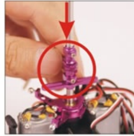
3. 下中心座组装入主轴 Install the bottom central holder set onto the main axle.
