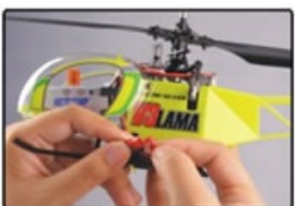
4. 接通电源 Connecting battery
