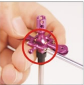
13. 夹头片装上中心座组并用螺丝锁紧 Install the grip set on the central hub set and lock it up with screws.
